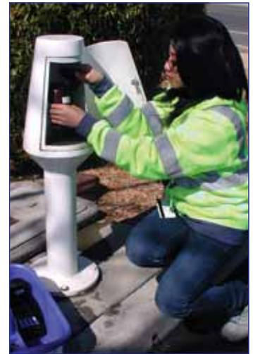
*Water samples collected at water quality sampling stations located throughout the Tri-City area are analyzed by ACWD's state certified laboratory chemists and technicians.*
